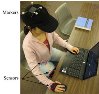
Fig. 2. Wireless motion sensor nodes worn on the human subject.
